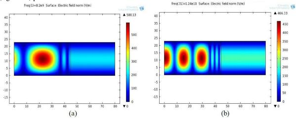
Figure 3: The calculated electric field distribution in the 2D case at 8.2 GHz (a) and 12.4 GHz (b). The DUT is just the jaw (pulp and bone, with  $\varepsilon_r$ =12)
