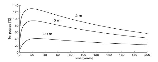
Figure 2: Temperature progression around the cylindrical canister. The distances from the axis of the cylinder are 2 m, 5 m and 20 m.
