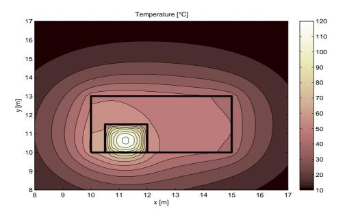
Figure 3: Temperature distribution around the canister in a vault one month after the installation. The temperature levels are scaled by 8 degrees.
