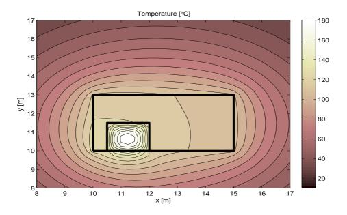
Figure 4: Temperature distribution around the canister in a vault six months after the installation. The temperature levels are scaled by 8 degrees.
