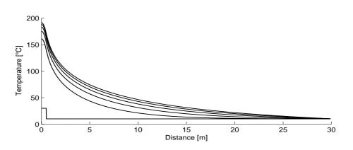
Figure 1: Temperature distribution around the cylindrical canister computed for 0, 1, 2, 3, 4 and 5 years after installation.
