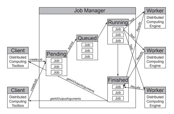
Figure 1: The priciples and architecture of the MATLAB Distributed Computing Toolbox and the Distributed Computing Engine
