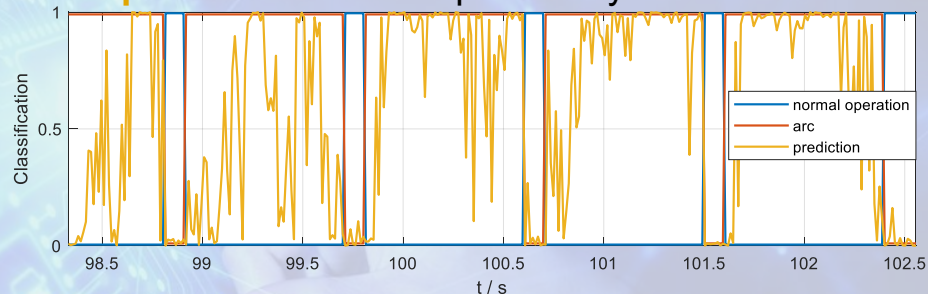
Output data: Predicted probability of an arc fault
