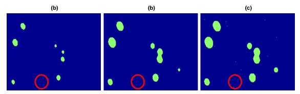
Figure 4: Threshold influence on object detection (a) detected objects T = 0.050, (b) detected objects T = 0.010, (c) detected objects T = 0.001.
