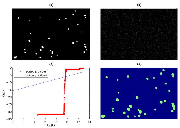
Figure 1: Model image object detection (a)model light image, (b)model dark image, (c) FDR evaluation, (d) detected objects in model image.
