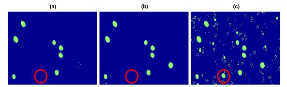
Figure 5: Object detection via. Laplacian of Gaussian (a) detected objects  $T_s = 10$ , (b) detected objects  $T_s = 5$ , (c) detected objects  $T_s = 1$ .
