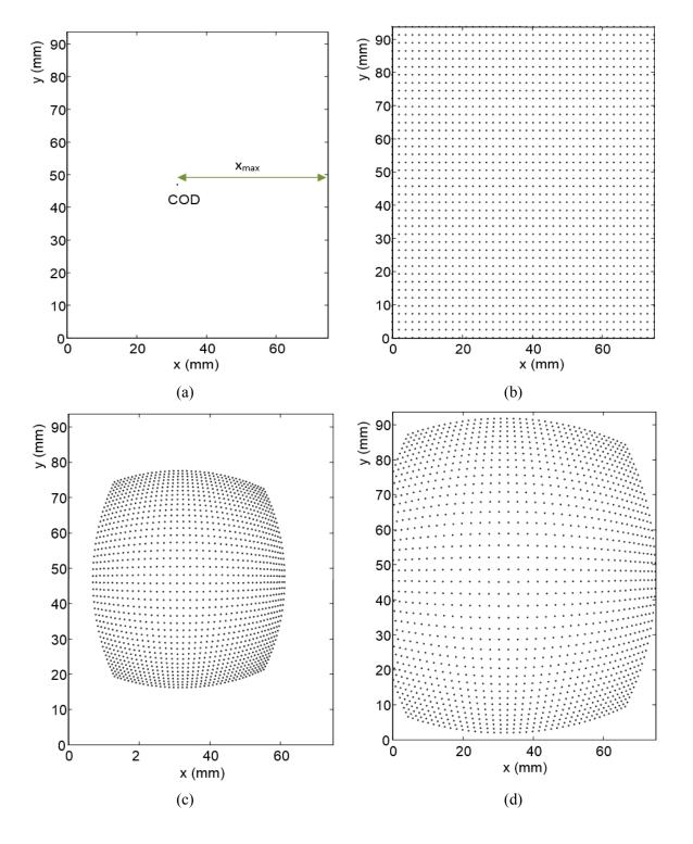
Figure 2 a) For description of COD and consecutive image transformation (b-d) needed for HMD devices.
