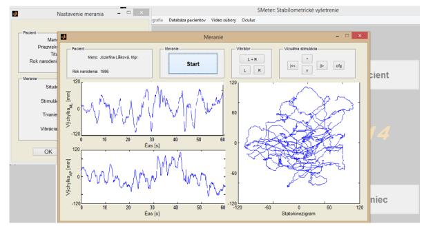
Figure 1. We developed Matlab based program that measure, acquire, analyze data as well as control visual stimulation – starts and stops it at the proper time
