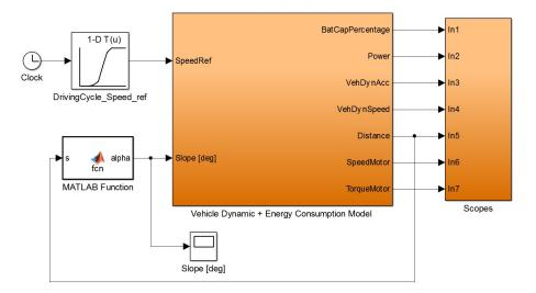
Figure 3: Whole model with inputs and outputs
