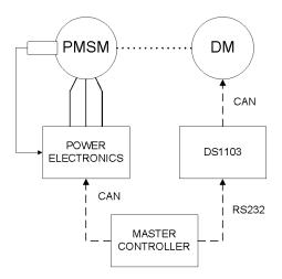
Figure 2: Hardware Structure of Laboratory Stand
