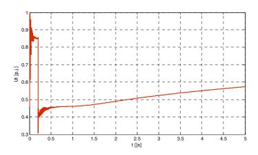
Figure 3: Diesel generator unit voltage response on load increase
