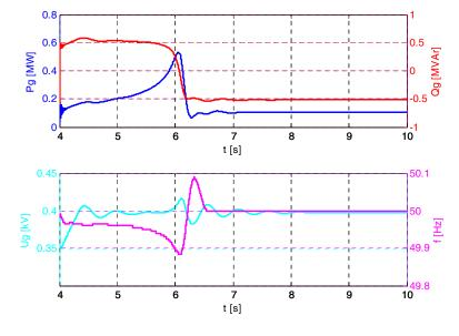
Figure 4: Diesel generator unit response on asynchronous motor switching
