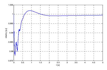
Figure 2: Diesel generator unit speed response on load increase
