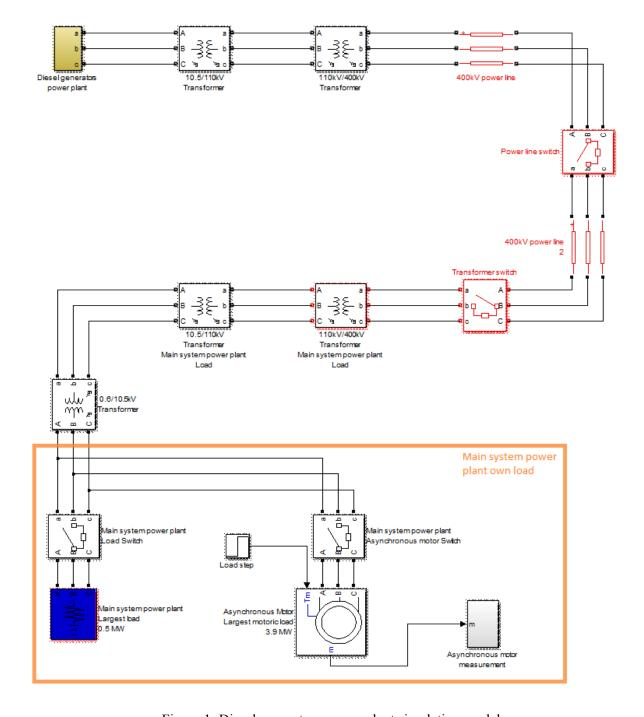
Figure 1: Diesel generators power plant simulation model
