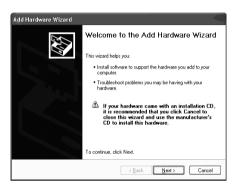
Insert installation floppy into drive a. In Found New Hardware Wizzard select Install the software automatically and click Next.
